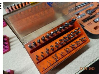
**169 1 x BohrerKassette 1,0-13,0 mm**
