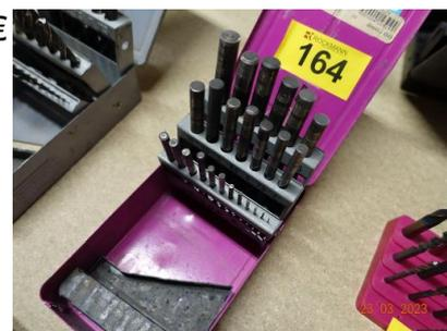
**165** 1 x **Bohrerkassette 1,0-13,0 mm**
